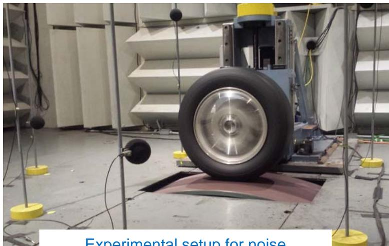
Experimental setup for noise measurement (Bridgestone Americas)
